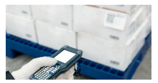
Barcode scanners need a direct line of sight to the label for accurate reading and decoding, so fogging or condensation on the scanner optics can present a problem. The best solution is to have the barcode reader integrated as a component of the handheld computer, to take advantage of the computer's internal heater to function properly.
