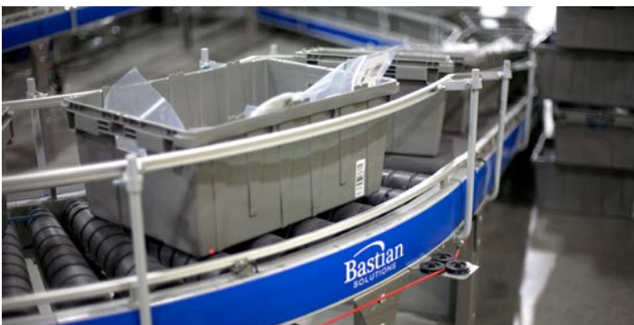
Even at an entry-level price point, conveyors make use of photo eyes and individually-driven conveyor zones to accomplish zero pressure accumulation.
