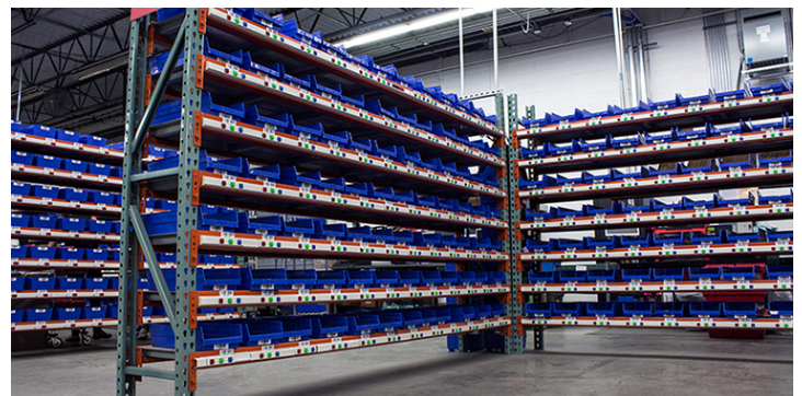
Put wall applications decouple the picking and packing process of order fulfillment maximizing the efficiency of each application.
