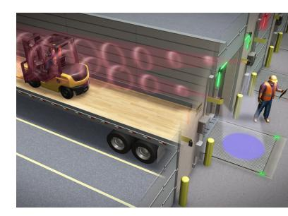
Corner-Vu<sup>™</sup> – With the Corner-Vu system, loading dock personnel will no longer have to guess whether or not a trailer is secured at the loading dock. Bright lights mounted on the inside top corners of the loading dock door indicate whether or not a trailer is properly secured. Green lights mean a trailer is safely secured and ready to enter, while red lights caution workers to stay clear. Visual status is also displayed on the Dok-Commander control system (lights and video display).
