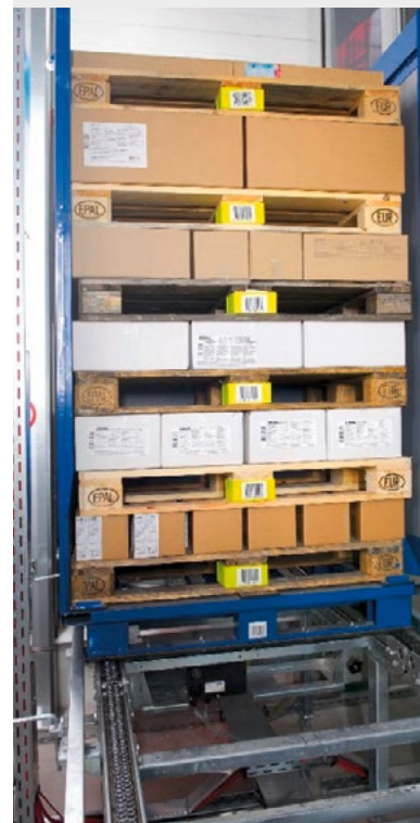
Store pallets: Consolidated fully automatically based on the respective store layout. (Image: WITRON)
