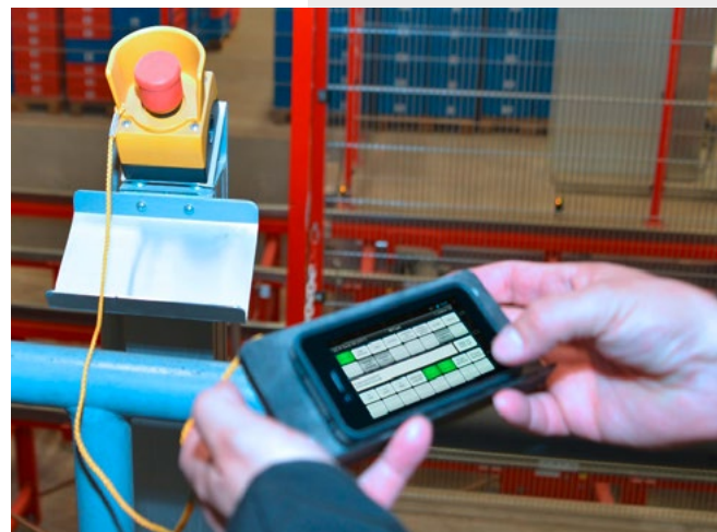
Modern system service: Direct machine communication via smart phone. (Image: WITRON)
