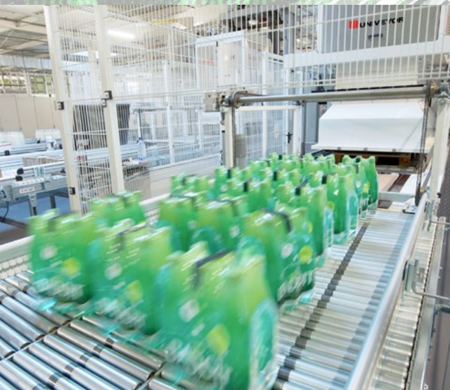
Communication of SKU to machine: The conveyor system adapts its speed automatically to the individual product. (Image: WITRON)
