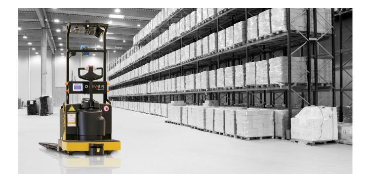
Additionally, robotic lift trucks comply with ANSI standards, abide by posted speed limits and follow site-specific safety protocols. They can stop and adjust to unexpected obstructions, including ground level impediments or obstacles suspended in midair, like a ladder sticking out of a storage area.
